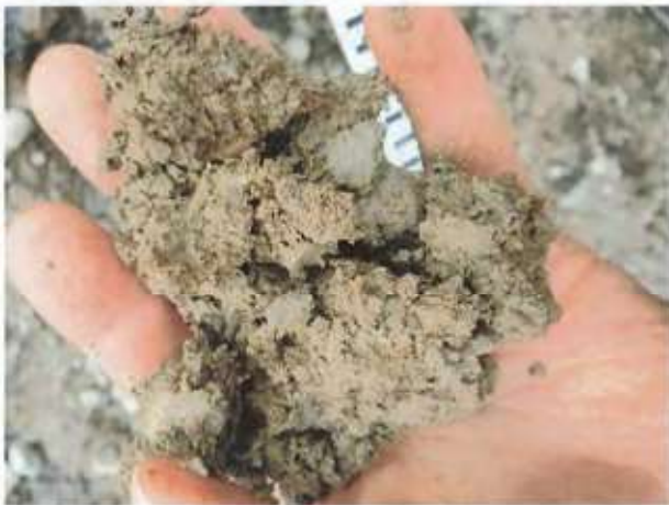
Peat and till exposed at new access track and drainage associated with ongoing forestry activities observed during site surveys 16/06/2020.
