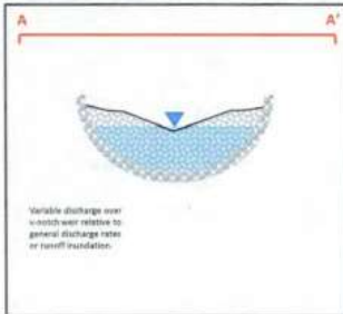
Constructed Drain and Check Dams – Section A-A'
